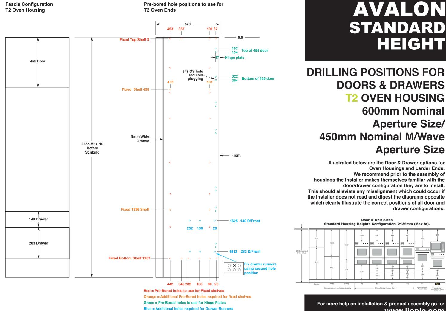
All positions shown are taken from 0.0 and should be reduced in accordance with any scribing, or marked up prior to assembly
