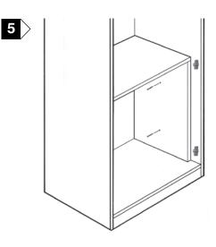
robe ensuring it is fully pressed home against back Both end panels require to be secured to robe end panels with screws provided It is left for installer to decide on position were holes are to be drilled for screws to be secured.
