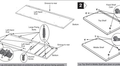
Lay Top Shelf & Middle Shelf face down on protective surface (with groove in Top Shelf facing upwards). Firmly press home Fixed Shelf Cams into pre-bored holes ensuring
