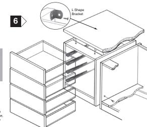
2 x 'L' shaped brackets are supplied for securing unit to wall or securing worktop to unit. If using brackets to secure worktop these will be placed in front of back panel. If using brackets to secure to wall position as indicated. Screws cannot be provided for securing to wall due to differing wall constructions.
