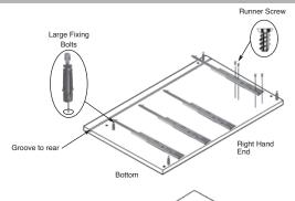
Bring all rails into position and secure to end panel as shown. Ensuring all Mini-fix cams are locked fully. Bring left hand end panel into position and secure to rails ensuring Mini-fix cams are locked fully
