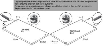
As the end panels are universal it is only required for mini-fix cams and wooden dowels to be
