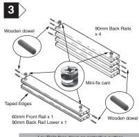
Lav Rails face down on protective surface. Firmly press home Mini Fix Cams into pre-bored holes ensuring arrow on cam faces outwards. Firmly press home wooden dowels into pre-bored holes, ensuring they are fully knocked in. NB: All back rails and back rail lower are 90mm deep, the front rail is 60mm deep. Always ensure the
