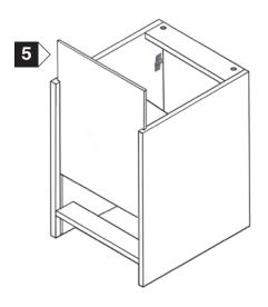
Bring unit into upright position and locate back panel into grooves in end panels.
