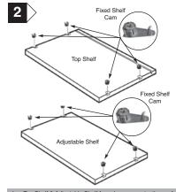
Lay Top Shelf & Adjustable Shelf face down on protective surface (with groove in Top Shelf facing upwards). Firmly press home Fixed Shelf Cams into pre-bored holes ensuring opening in cams face outwards As an option additional adjustable shelves can be purchased to
