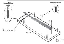
3 Bring top & bottom shelves into position and secure to end panel as shown. Ensuring all Mini-fix cams are locked fully. NB. Ensure grooves in
