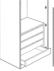
position and place on to fully extended runners. Ensure drawer runner locates into the rear of the drilled hole). Firmly close the drawer into the unit. The drawer should locate onto the runner. Repeat this action with each drawer. If drawer fascia adjustment is required. slacken drawer fascia retaining screws. Within the drawer front adjuster there is a floating mechanism which allows for 2mm adjustment in two directions. Adjust as necessary and tighten drawer fascia retaining
