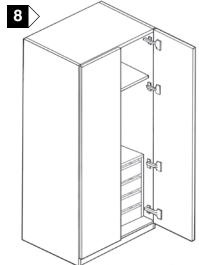
Once adjustable shelf has been placed into position, secure hanging rail support to end panels and place hanging rail into position. Bring door/s into position and place onto hinge plates, lock into position by firmly pressing arm on hinge home.
