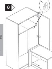
Once adjustable shelf has been placed into position, secure hanging rail support to end panels and place hanging rail into position. Bring door/s into position and place onto hinge plates lock into position by firmly pressing arm on hinge Adjust as shown in diagram
