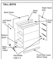
Lay end panels face down on protective surface with groove facing upwards. Fix Large Fixing Bolts into positions indicated. Bring Drawer runners into position and fix to end panels into pre-bored holes with runner screws.
