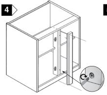
Bring corner post into position and secure to inner corner post as shown. Ensuring all Mini-fix cams are locked fully. As the internal space is reduced by the internal corner post the adjustable shelf will require scribing around the internal corner post, once this has been completed bring adjustable shelf into position and fully press down onto Mini-fixing bolts. Fully lock all Fixed shelf cams.
