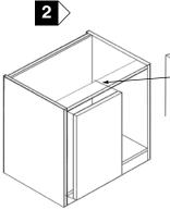
As there are multiple options of door size that can be used for the corner base, it will be required for installer to mark the position where the inner corner post is to be fitted. When the handing of the corner base has been decided bring door into position against base ensuring the door is flush with
