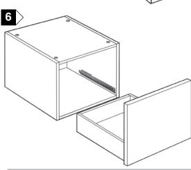
Once drawer front is fitted to drawer box bring drawer into position and place onto fully extended runners. Ensure drawer runner locates into the rear of the drawer box (small pre drilled hole). Firmly close the drawer into the unit. The drawer should locate
