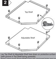
Firmly press home Fixed Shelf Cams into pre-bored holes ensuring opening in cams face outwards
