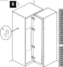
support to end panels and place hanging rail into position. Bring door into position and place onto hinge plates, lock into position by firmly pressing arm on Adjust as shown in diagram opposite.
