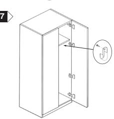
Once adjustable shelf has been placed into position, secure hanging rail support to end panels and place hanging rail into position. Bring door/s into position and place onto hinge plates, lock into position by firmly pressing arm on Adjust as shown in diagram opposite. If required the unused pre-bored holes in end panels can be plugged with the 5mm cover caps supplied.
