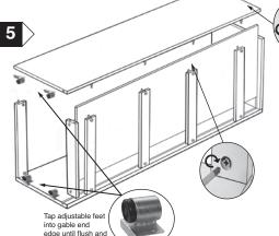
Bring back panel into position and locate into grooves in end panel and top shelf. Bring other end panel into position and place onto all rails, back panel and top shelf, ensuring all cams & dowels are located correctly Fully lock all Mini-fix cams & Fixed shelf cams.
