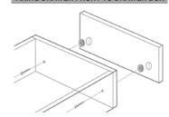
Firmly press drawer front adjusters into prebored holes in drawer front, bring drawer box into position and secure to drawer front with screws provided through pre-bored holes in drawer box.
