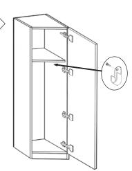
Once adjustable shelf has been placed into position, secure hanging rail support to end panels and place hanging rail into position. Bring door into position and place onto hinge plates, lock into position by firmly pressing arm on hinge home. Adjust as shown in diagram opposite. If required the unused pre-bored holes in end panels can be plugged with the 5mm
