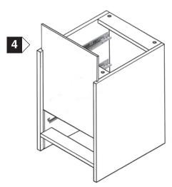
Bring unit into upright position and locate back panel into grooves in end panels.
