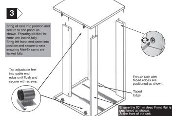
Lay Rails face down on protective Firmly press home Mini Fix Cams into pre-bored holes ensuring arrow on cam faces outwards. Firmly press home wooden dowels into pre-bored holes, ensuring they are fully knocked in. NB: Back rail, front rail and back rail lower are 90mm deep, the front rail lower is 60mm deep. Always ensure the front rail is placed in the correct position when assembling.
