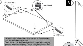
Firmly press home wooden dowels into pre-bored holes, ensuring they are fully knocked in.
