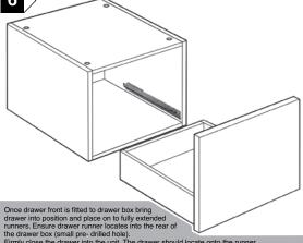
Firmly close the drawer into the unit. The drawer should locate onto the runner. If drawer fascia adjustment is required, slacken drawer fascia retaining screws. Within the drawer front adjuster there is a floating mechanism which allows for 2mm adjustment in two directions. Adjust as necessary and tighten drawer fascia retaining screws.
