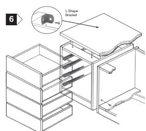
2 x 'L' shaped brackets are supplied for securing unit to wall or securing worktop to unit. If using brackets to secure worktop these will be placed in front of back panel. If using brackets to secure to wall position as indicated. Screws cannot be provided for securing to wall due to differing wall constructions
