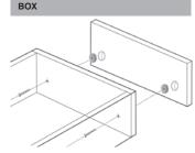
Firmly press drawer front adjusters into prebored holes in drawer front, bring drawer box into position and secure to drawer front with screws provided through pre-bored holes in drawer box
