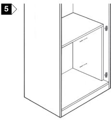
robe ensuring it is fully pressed home against back Both end panels require to be secured to robe end panels with screws provided It is left for installer to decide on position were holes are to be drilled for screws to be
