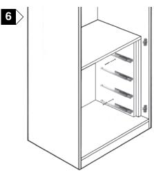
nto position against unit end panels. Both end panels with drawer runners fitted require to be secured to unit end panels with screws t is left for installer to decide on position were holes are to be drilled for screws to be secured.
