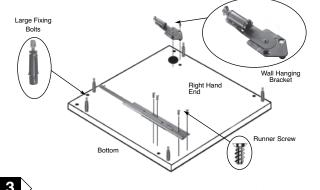
3 Bring top & bottom shelves & back rail into position and secure to end panel as shown. Ensuring all Mini-fix cams are locked fully.
