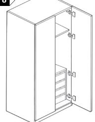
position, secure hanging rail support to end panels and place hanging rail into position. Bring door/s into position and place onto hinge plates, lock into position by firmly pressing arm on hinge home. Adjust as shown in diagram opposite. If required the unused pre-bored holes in end panels can be plugged with the 5mm cover caps supplied.
