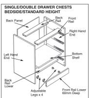
Lay end panels face down on protective surface with groove facing upwards. Fix Large Fixing Bolts into positions indicated. Bring Drawer runners into position and fix to end panels into pre-bored holes with runner screws. Repeat operation for Left hand end panel.
