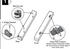
Lay inner corner post face down on protective surface with pre-bored holes facing upwards, firmly press home into holes Mini Fix Cams ensuring arrow on cam faces outwards.
