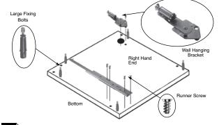
Lay end panels face down on protective surface. Fix Large Fixing Bolts into positions indicated. Bring Drawer runner into position and fix to end panel into pre-bored holes with runner screws. Bring Wall hanging bracket into position, firmly press home into pre-bored holes, secure with Repeat operation for Left hand end panel.
