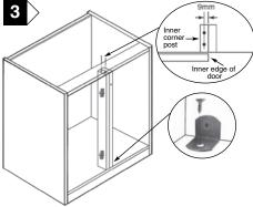
two pre bored holes will be required to be drilled through the front rail by the installer in suitable positions, secure post to top rail with 45mm screws provided. Secure bottom of post to bottom shelf through 'L' shape brackets with screws provided.
