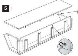
Bring back panel into position and locate into grooves in end panel, top and bottom shelves Bring other end panel into position and place onto all rails, back panel, top and bottom shelves, ensuring all cams & dowels are located Fully lock all Mini-fix cams &
