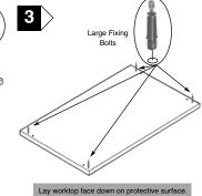
Fix Large Fixing Bolts into positions indicated.
