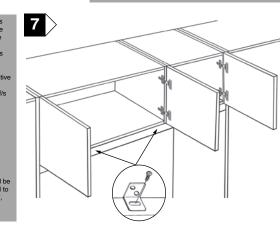
If fitting the OPTIONAL PELMET, fit metal brackets (not supplied) to rear of pelmet prior to fitting to bridging cupboards. Bring door/s into position and place onto hinge plates, lock into position by firmly pressing arm on hinge
