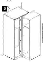
Place unit into position were it is to be located. Ensuring gap to wall is correct to size of door being used, (see diagrams below for spacing details) Bring adjoining unit into position as shown and secure to corner post with suitable size screws.
