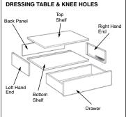
Lay end panels face down on protective surface with groove facing upwards. Fix Large Fixing Bolts into positions indicated.
