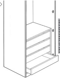
Once drawer fronts are bring drawers into position and place onto fully extended runners. Ensure drawer runner locates into the rear of the drawer box (small predrilled hole). Firmly close the drawer into the unit. The drawer should locate onto the runner Repeat this action with each drawer.
