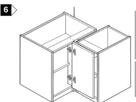
Bring door into position and place onto hinge plates, lock into position by firmly pressing arm on hinge home. Adjust as shown in diagram opposite. If required the unused pre-bored holes in end panels can be plugged with the 5mm cover caps
