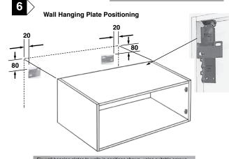
Fix wall hanging plates to walls in positions shown, using suitable screws, these are not provided because of differing wall construction. Bridging cupboards can be sited in multiple locations, if they are to be sited between robes always ensure robes are correctly levelled in all plains prior to bridging cupboard/s being installed. For adjustment of wall hanging brackets see diagrams opposite.
