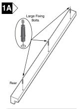
surface with pre-bored holes facing upwards. Fix Large Fixing Bolts into positions indicated.
