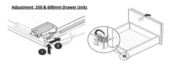
Height - Push grey lever up, then back. The further you push back, the higher the front rises (0 - 3mm) Tilt - Twist cam at rear to achieve tilt of front (would normally only apply to very high fronts)
