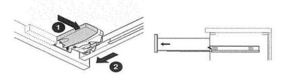
Insertion - Keep drawer base square to runner & push back, it will automatically lock in place.
