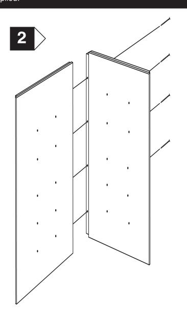
Bring back panels into position and secure with 45mm construction screws provided. It is essential that back panels are fitted correctly with all pre bored holes in alignment.
