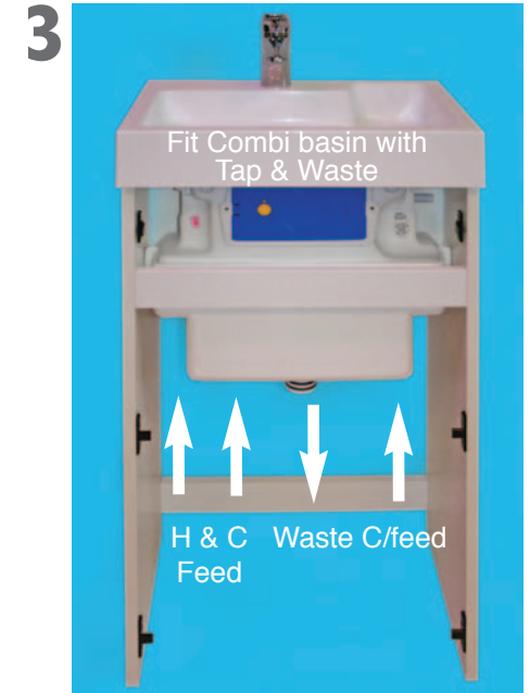
Plumb & fit basin with taps. Note: If a Sensor tap is used, ensure the battery pack is positioned in front of cistern support rail to allow for easy battery replacement in the future.
