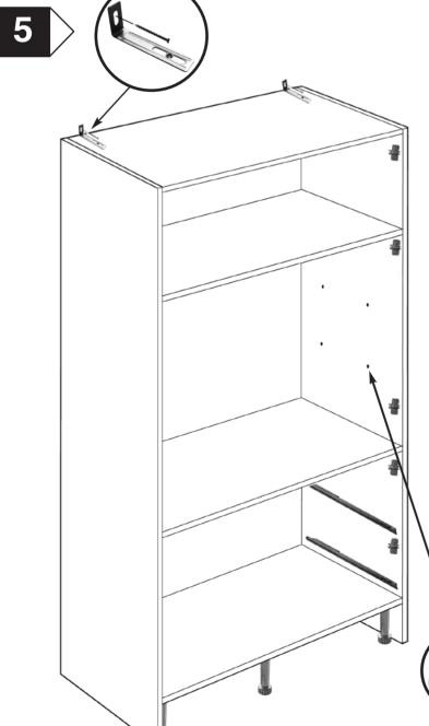
Bring unit into position were it is to be fitted and level in all plains, place 'L' shape brackets provided onto top shelf and Secure unit to wall, screws cannot be provided because of differeing When unit is securely fitted in position firmly push shelf supports into pre-bored holes in end panels. IMPORTANT. When adjusting the height of the unit make sure that the legs are not adjusted below the nominal 140mm plinth height.
