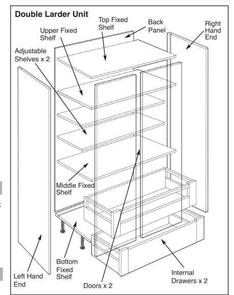
Note:It is strongly recomended that the unit is secured to the wall prior to Doors, drawers & adjustable shelves being fitted.
