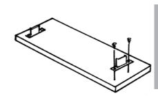
Starter holes for fixing drawer bracket to drawer front are provided on the rear of all drawer fronts.
