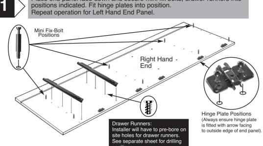
Place end panel face down and secure mini fix bolts, drawer runners into
